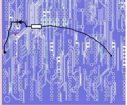
Now there are 3 additional resistors of 470 Ohm and 2 diodes 1N4148 inserted for the addressing of the sound chip..
