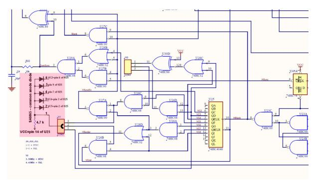
311 lines mod: for the diode SAM65 see <u>www.ebay.de/itm/271413514510</u> or use D7-1A from farnell uk.farnell.com/bi-technologies-tt-electronics/d71a/diode-network-bussed/dp/1689663?ost=D71a or 5 single diodes (1N4148)
