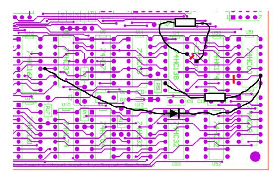
At the bottom side cut the connection that comes from pin 11 of U51. Insert a resistor of 470 in series to that line and insert a diode 1N4148 – cathode at the side of the new resistor that is not on pin 11 of U51 (signal BDIR) and anode at pin 5 of U5 (signal /RD).
